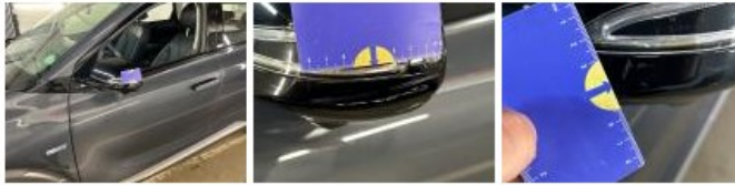
Outside rear-view mirror housing L, Broken, Replace
