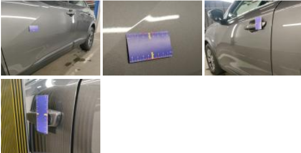
Central pillar L, Dent(s) and scratch(es), Spot repair
