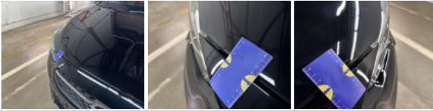
Bonnet, Dent(s) and scratch(es), Spot repair
