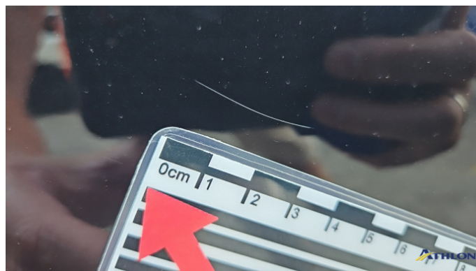
6. Tür Hinten - Links Kratzer
