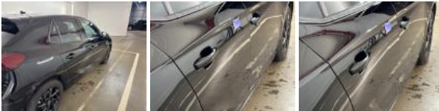
Door FR, Bad repair, Spot repair
