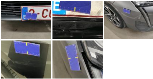
Grille, Broken, Replace
