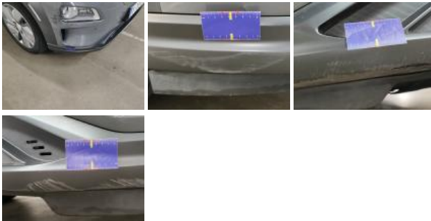
Bumper grille, Crack, Replace
