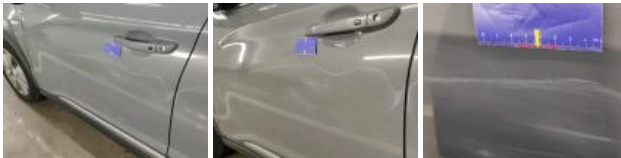
Door RL, Scratch(es), Repair and paint (complete)
