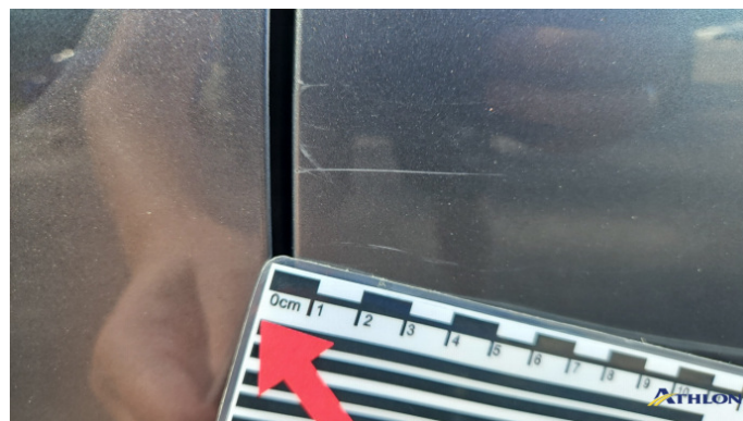
3. Tür Hinten - Links Kratzer
