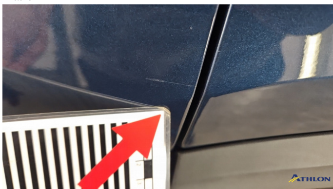
4. Tür Hinten - Links Kratzer
