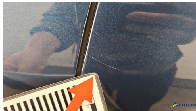
4. Tür Hinten - Links Kratzer
