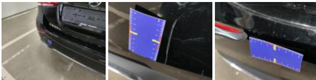
Sill trim R, Dent(s) and scratch(es), Repair and paint (complete)
