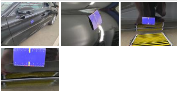
Door RL, Dent(s) and scratch(es), Spot repair
