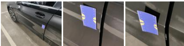
Central pillar L, Dent(s) and scratch(es), Spot repair
