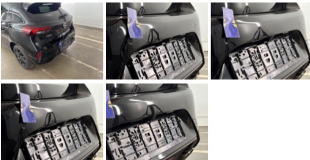
Door RR, Dent(s), Paintless dent repair
