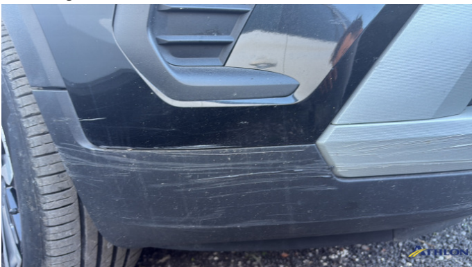
6. spoiler anteriore 3 ammaccature
