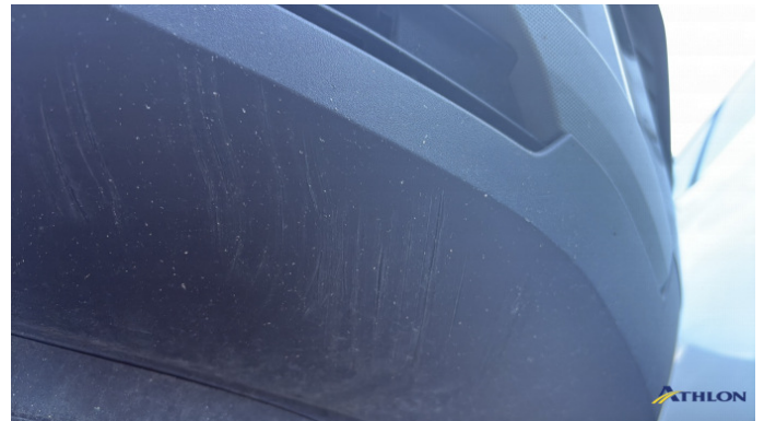
6. spoiler anteriore 3 ammaccature
