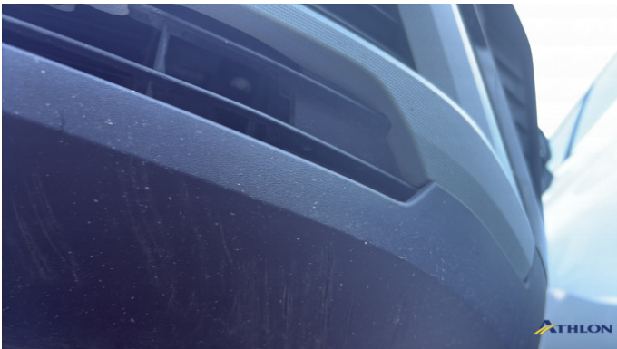
6. spoiler anteriore 3 ammaccature
