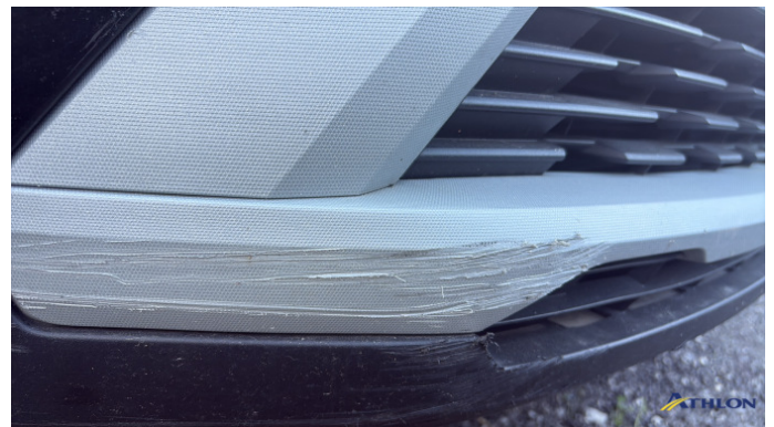
6. spoiler anteriore 3 ammaccature
