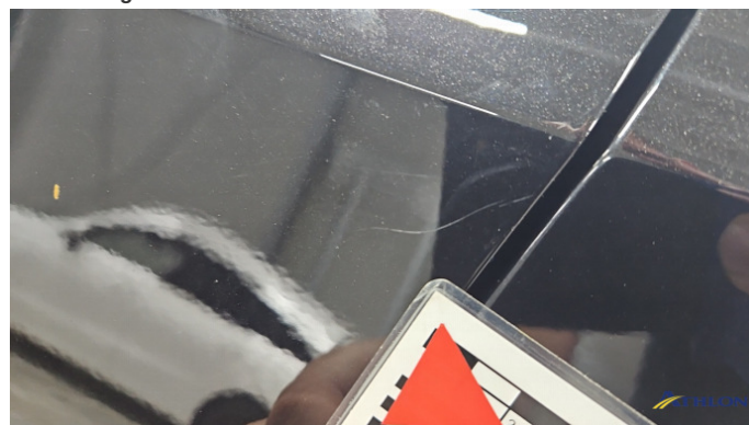
5. Tür Vorne - Links Kratzer
