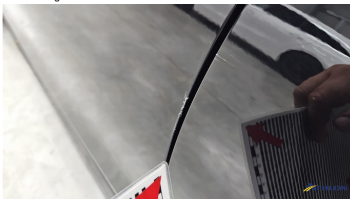
5. Tür Vorne - Links Kratzer
