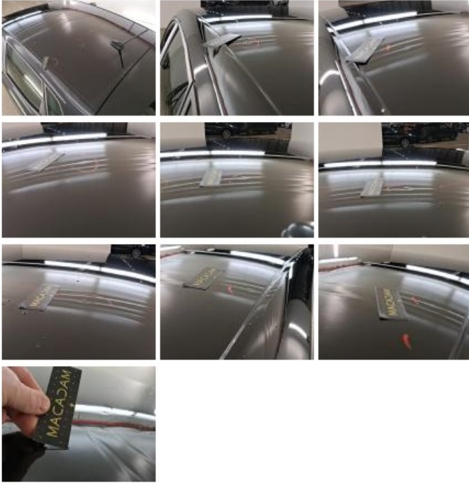
Roof, Dent(s), Paintless dent repair
