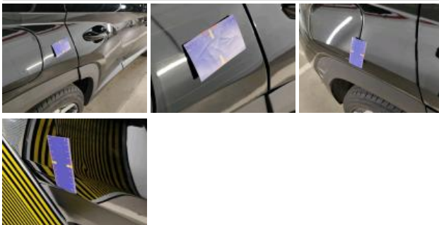
Door trim RR, Deformed / Strained, Replace
