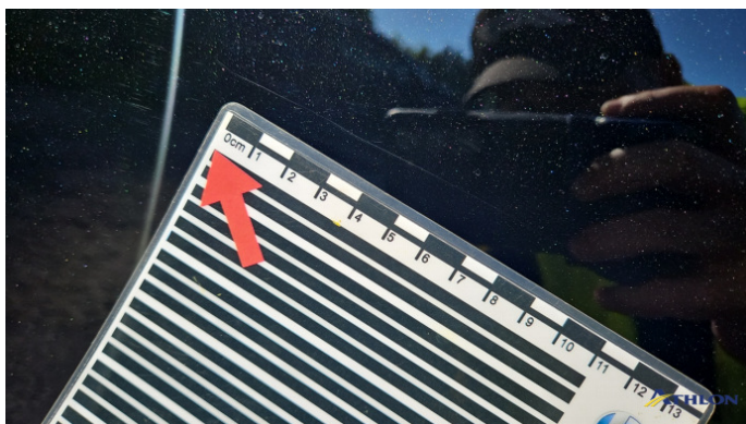
3. Tür Hinten - Links Kratzer
