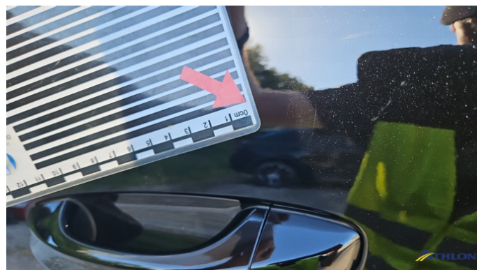
2. Tür Vorne - Links Kratzer
