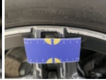
Alloy rim RL polished, Scratch(es), Repair and paint (complete)
