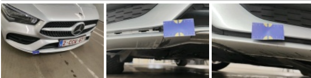
Bumper F, Scratch(es), Repair and paint (complete)
