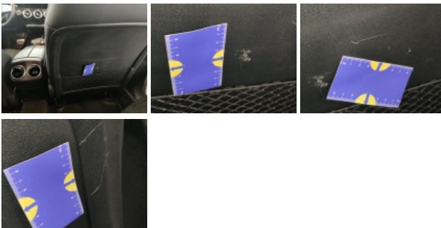
Floor covering FR, Burned, Smart repair
