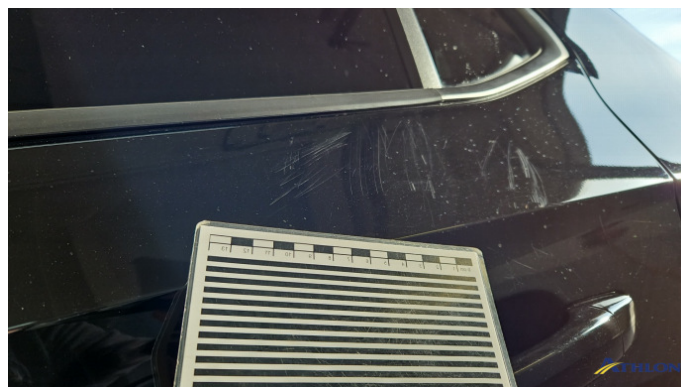
2. Tür Hinten - Links Kratzer Ab 60mm
