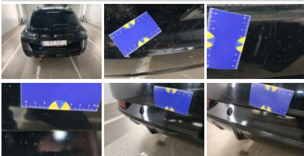
Bumper R, Scratch(es), Repair and paint (complete)
