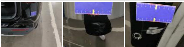
Bumper R, Broken, Replace
