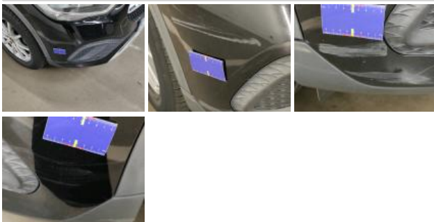
Bumper moulding F, Scratch(es), Replace
