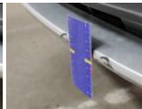
Bumper moulding F, Dent(s) and scratch(es), Replace
