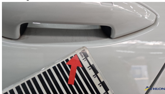
7. Tür Hinten - Links Kratzer
