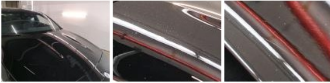
Windscreen moulding, Damaged, Replace
