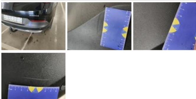
Wheel arch cover FR. Deformed / Strained. Replace
