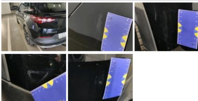
Bumper moulding R, Scratch(es), Smart repair
