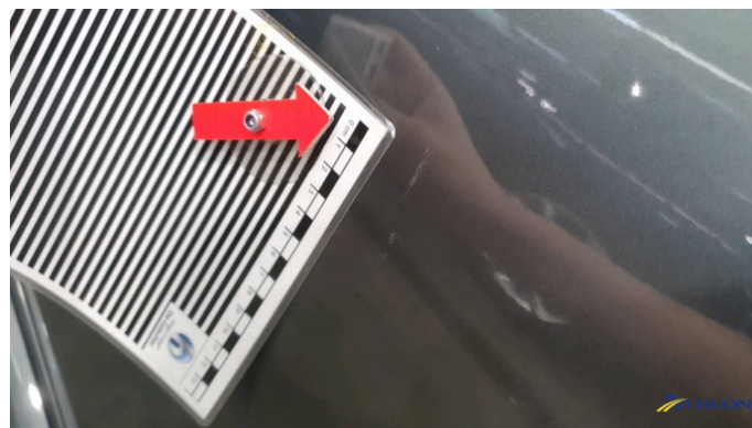
4. Tür Vorne - Links Kratzer
