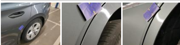
Wing RL, Bad repair, Spot repair
