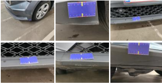
Bumper F, Crack, Replace and paint
