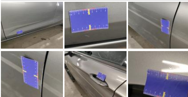
Door RL, Scratch(es), Spot repair
