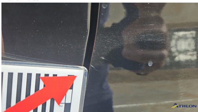
6. Tür Hinten - Links Kratzer
