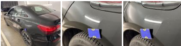
Door RL, Dent(s) and scratch(es), Spot repair
