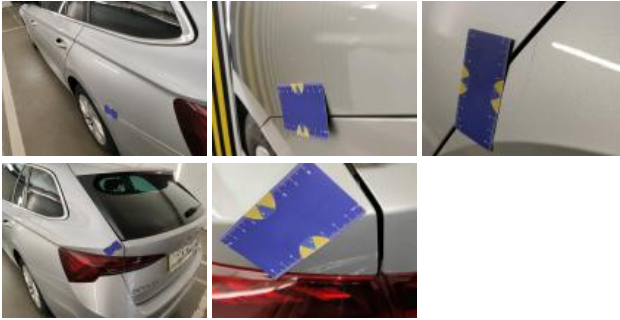
Door RL, Dent(s) and scratch(es), Spot repair
