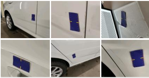
Outer door handle RR, Scratch(es), Repair and paint (complete)
