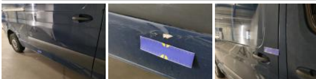
Sliding door R, Scratch(es), Spot repair
