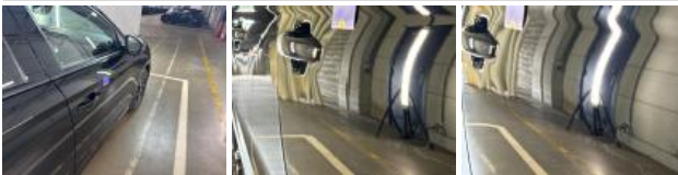
Wing FR, Bad repair, Spot repair
