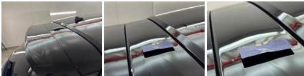
Outside rear-view mirror housing R, Scratch(es), Acceptable
