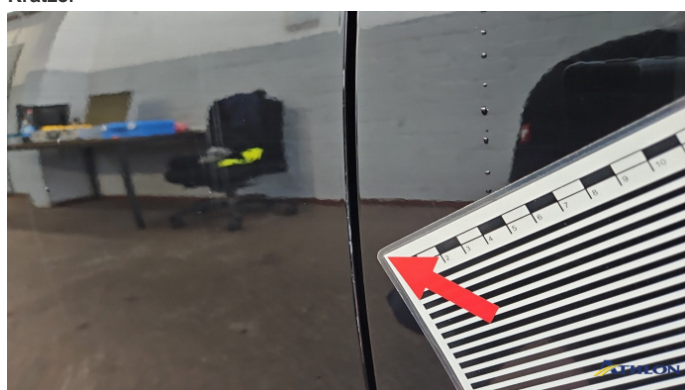
3. Tür Vorne - Links Kratzer
