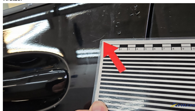
3. Tür Vorne - Links Kratzer
