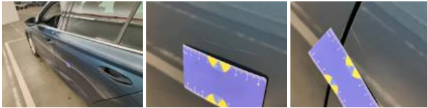
Door FL, Dent(s) and scratch(es), Spot repair
