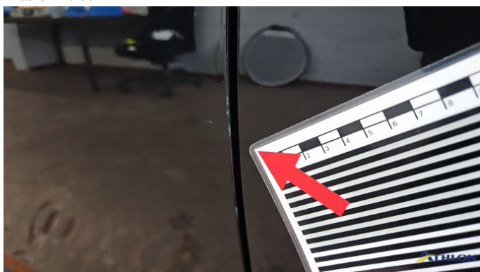
2. Tür Vorne - Links Kratzer
