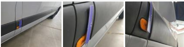
Mirror side repeater L, Deformed / Strained, Replace
