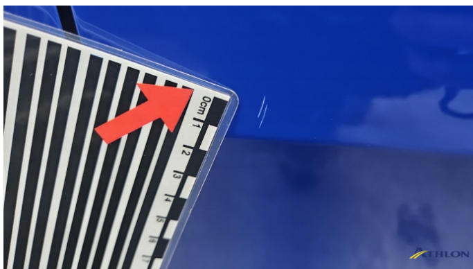
7. Tür Hinten - Links Kratzer Ab 60mm
