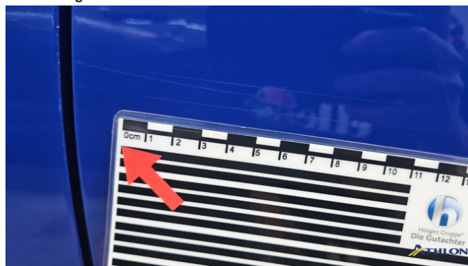
7. Tür Hinten - Links Kratzer Ab 60mm
