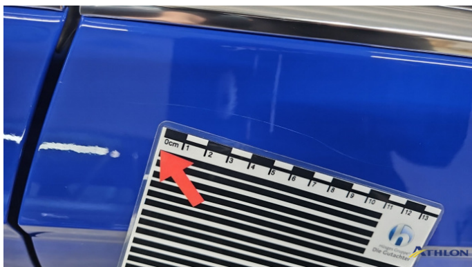
7. Tür Hinten - Links Kratzer Ab 60mm
