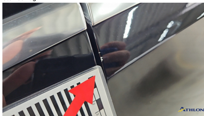
4. Tür Hinten - Links Kratzer
