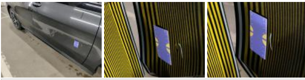
Roof pillar R, Scratch(es), Acceptable
