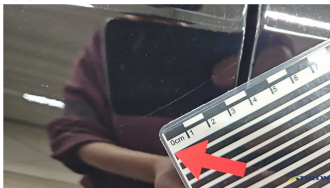
5. Tür Hinten - Links Kratzer
